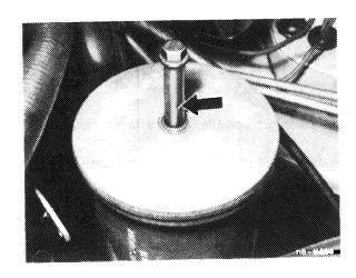
On 2nd version, unscrew oil filter cover and pull up for a short distance so that the oil can flow back to oil pan.
